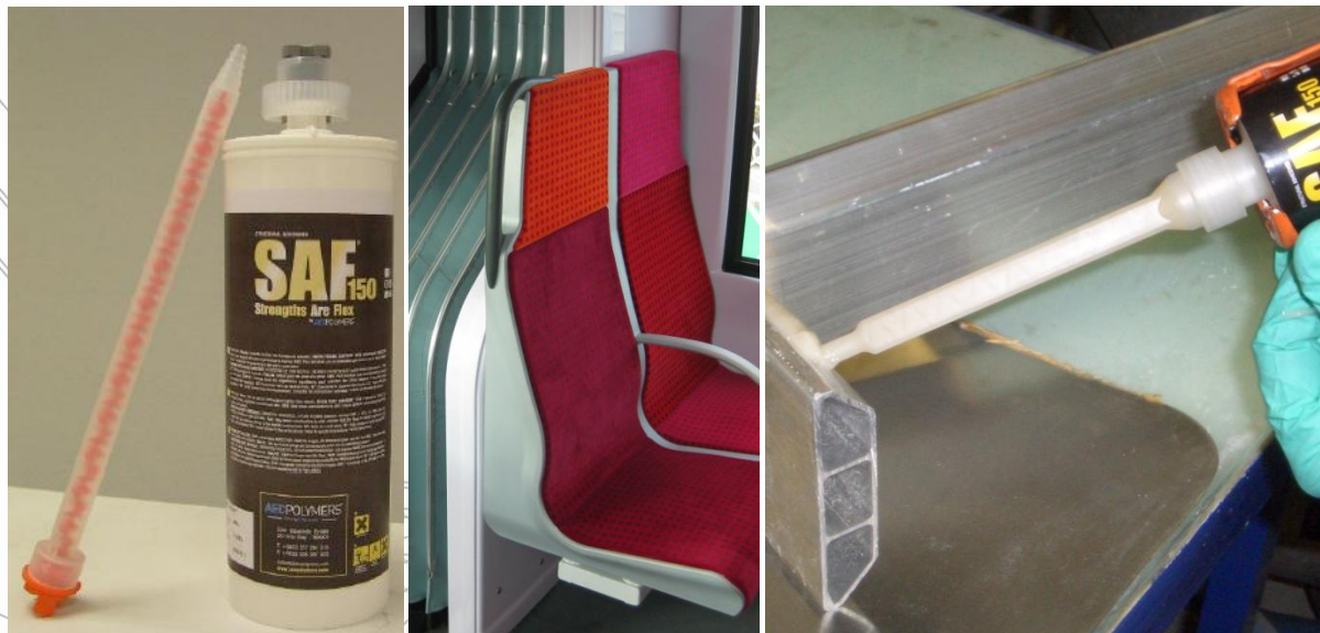
Structural seats assembly - Application on Aluminium (6060)
